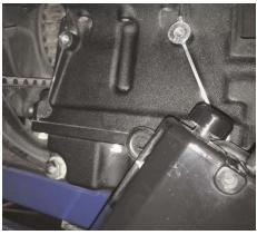
Attach the spoiler bracket as shown on the pictures below. The bracket should be underneath the evaporation system reservoir. If your motorcycle doesn't have the evaporation system just attach the bracket using the included bolts. Don't forget to use thread locker glue (not included).
