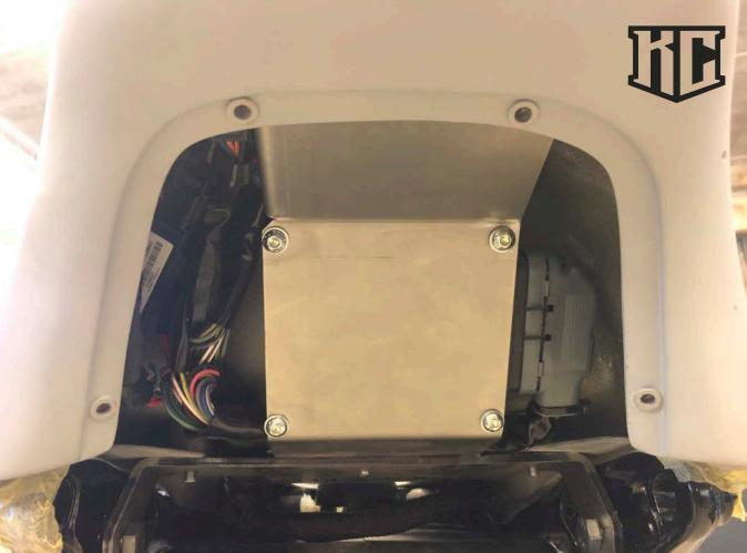
Place the wiring harness inside and fasten lower cover using four screws
