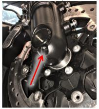
It is fixed using fixing screw. Use the thread locker glue (not included).
