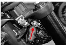
3. Attach the headlight grill as shown on the below picture. Use the included M6x16 bolts, M6 nuts and washers. See the picture below. Adjust the position of the grill.
