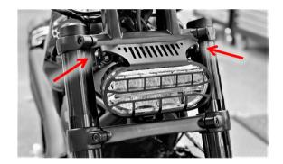
4. Adjust the headlight level if needed and the installation is complete.
