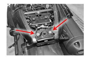
6. For rebuilding the wiring, you will need sharp, thin needle, or pick tool. The six-pin connector is located under the left side cover. Pull it to remove. Disconnect the connector and remove pins from the male side using a sharp needle or pick tool. Place your new tail light wiring and push pins in the connector. Refer to the table below. Rear light wiring color for DIY:
